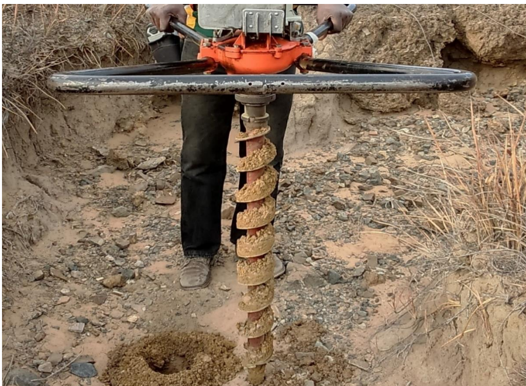
Figure 4.6: Drilling machine with a 1 m bit for collection of soils at different depths
