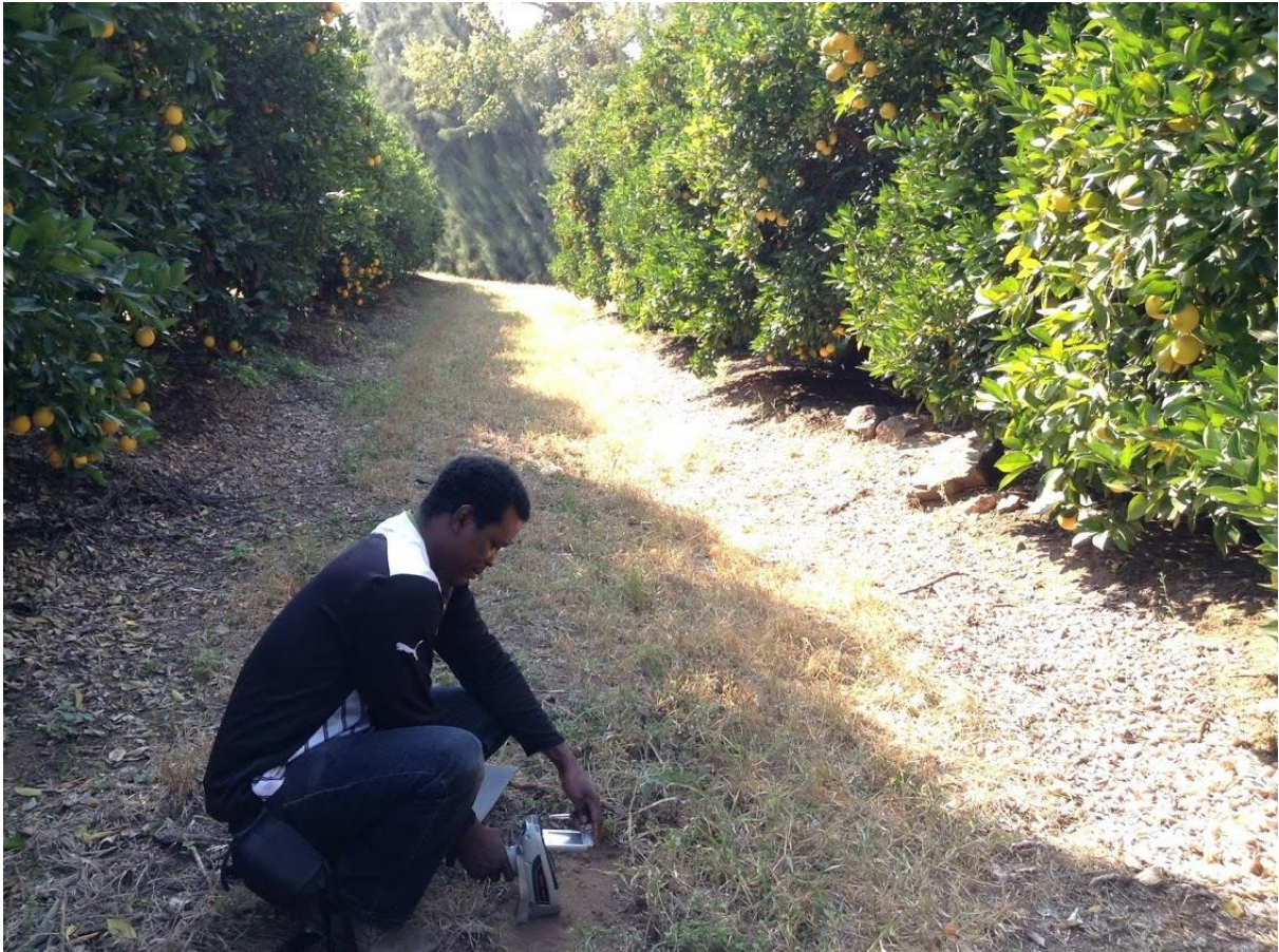
Figure 5.2: In situ analysis of soil between the rows of trees in a citrus orchard using the pXRF spectrometer
