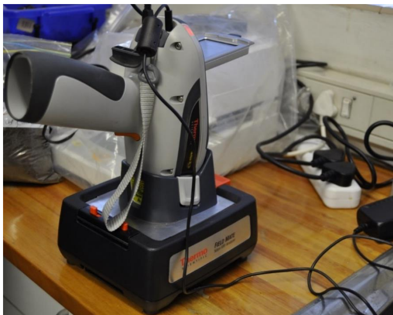
Figure 3.1: The Niton XL 3t GOLDD™+ spectrometer used in this study for the analysis of pelletized samples in the laboratory
