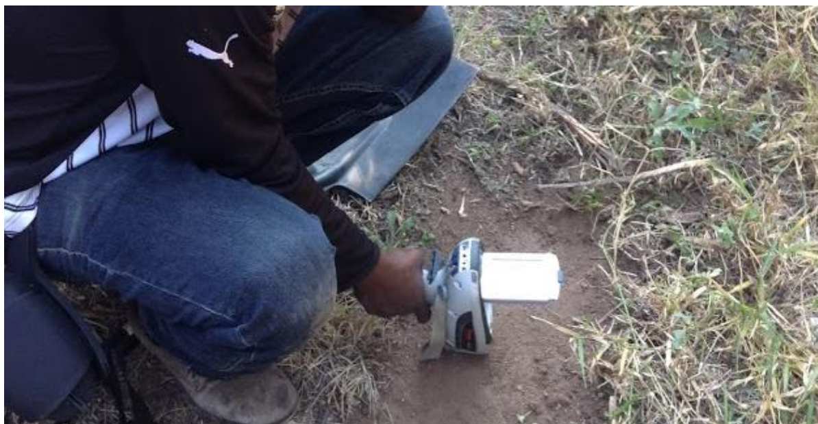
Figure 3.2: Field analysis of soil using the pXRF spectrometer
