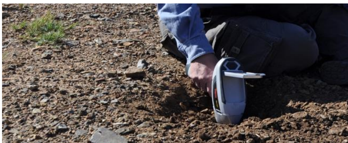
Figure 4.5: Measurement of metal concentrations in soil using the portable X-ray fluorescence spectrometer
